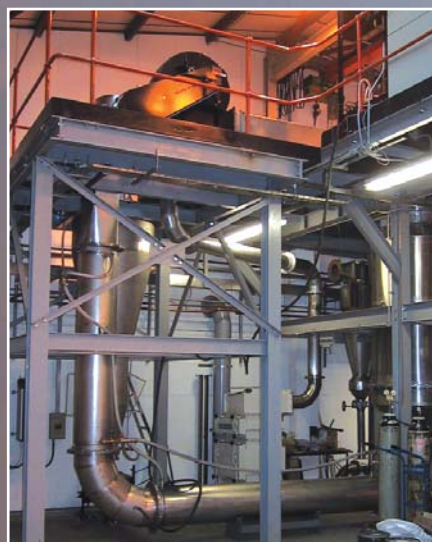
Fig.1 The Anti-Satellite system installed on ASL's gas atomiser
