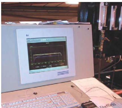
The PC/PLC control system that enables many parameters to be varied and monitored
