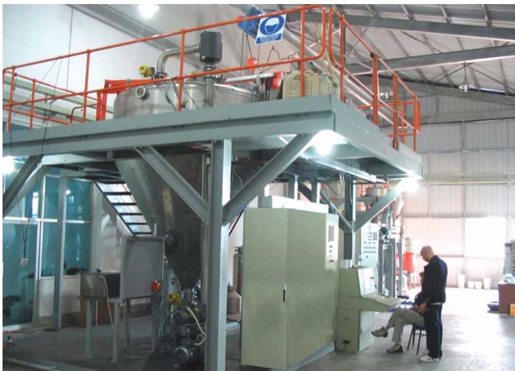
The centrifugal solder atomiser installed at the clients facility.
