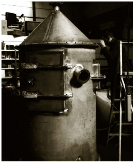
Water Atomiser for confidential client being assembled in Sheffield. Capacity up to 150kg/min of steel.
